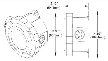
Figure 1: CO Sensor with optional Conduit Fitting
